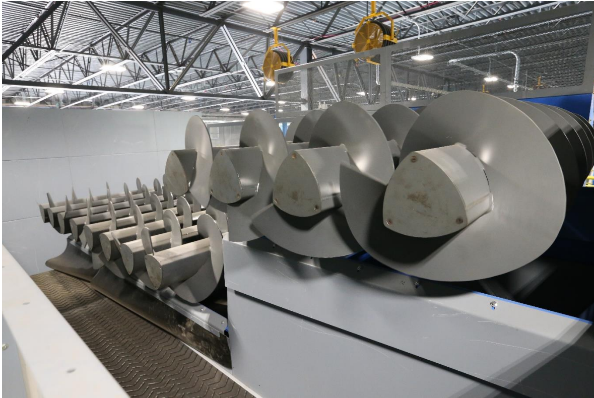
Figure 3: OCC Auger Screen's patented non-round design
