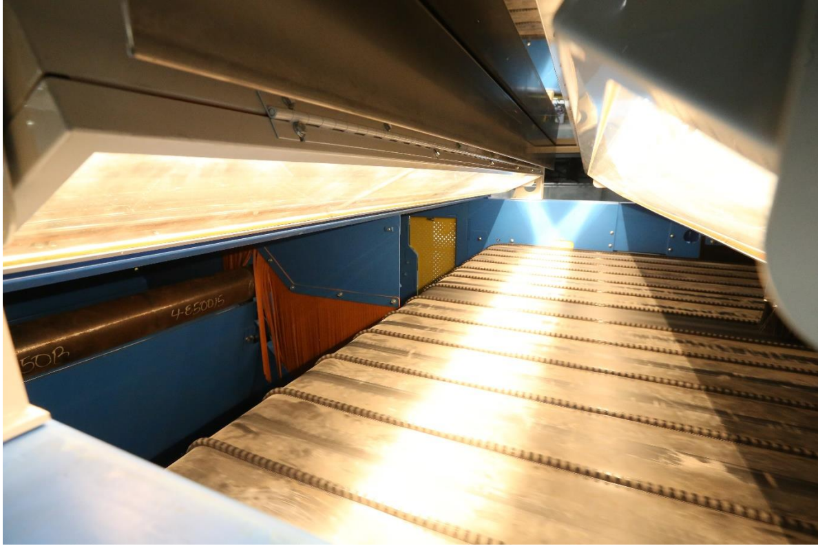
Figure 6: Optical sorters use lighting to identify and separate recyclables
