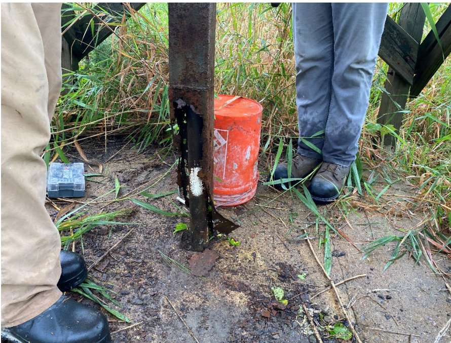
Photo 6: MW-17 protop prior to abandonment. Rusted out, did not require additional tools to remove. (Looking down)
