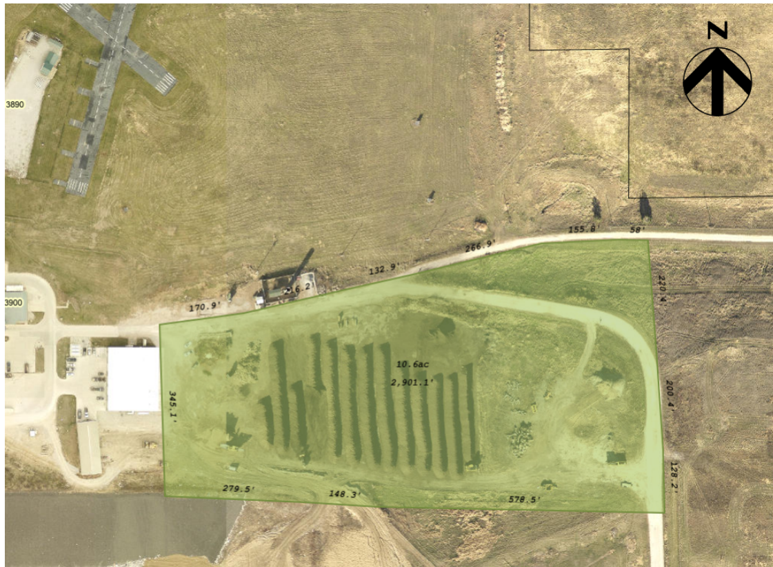
Figure 1. Limits of Excavation
