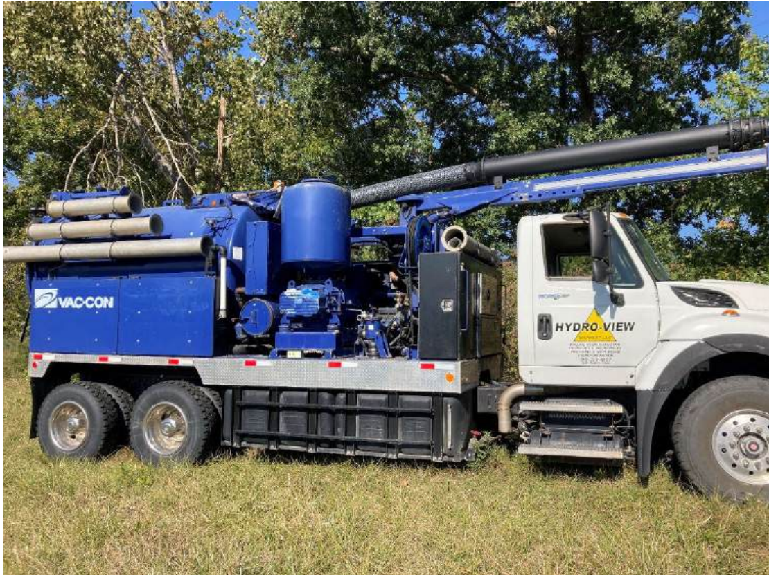
Hydro-View equipment used for jetting
