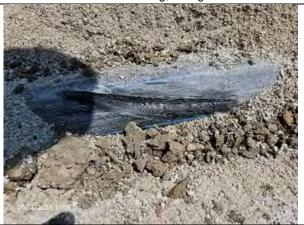
Damage on the existing 4-IN water main, facing east.
