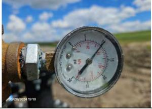
End of pressure test for 4-IN HDPE, facing south.
