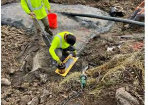
Vacuum box non-destructive testing by CEC on the completed extrusion welds, facing northeast.
