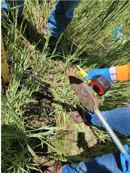
View of soil in boring with transition from vegetative cover to clay cap in auger.
