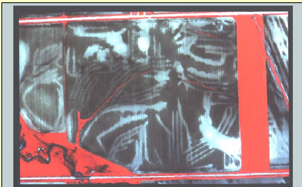
Figure 4. Using remote sensing, tile lines are indicated by lighter soil (active drainage), while darker (moist) soils indicate slower drainage.
