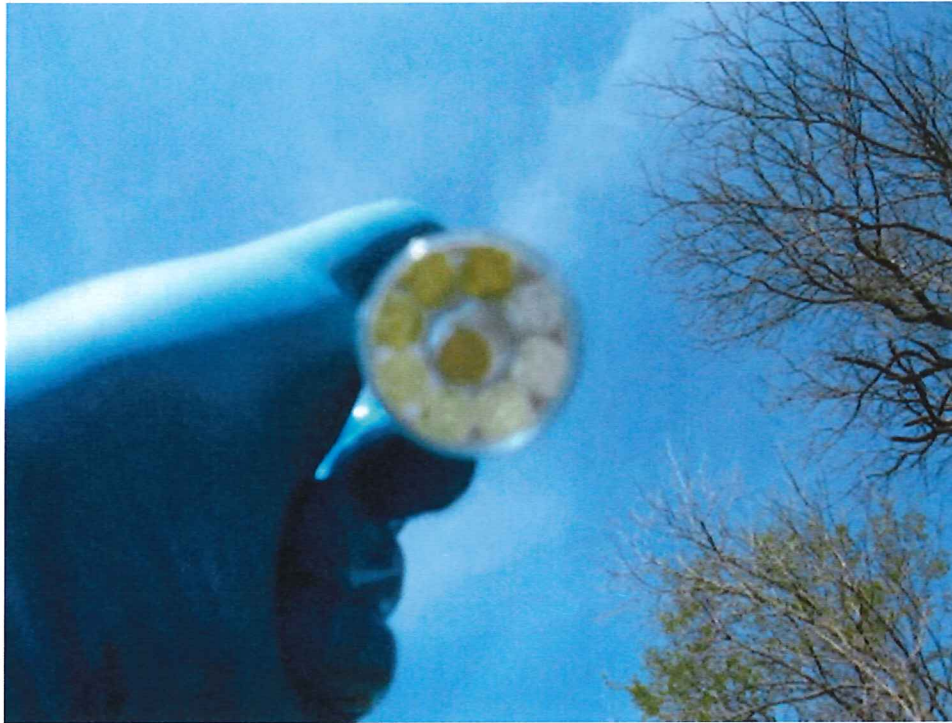
Above: The results of the low level ammonia field test kit from the ditch, showing approximately 1 ppm. Below: Looking upstream (west) from the road at the unnamed tributary.
