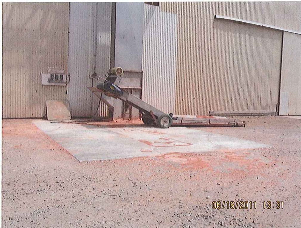
Above: Agriland catchment basin on June 16. Below: Dry fertilizer spilled on west side of dry fertilizer storage facility. Recommend a larger concrete pad to aid in cleanup of spilled fertilizer.
