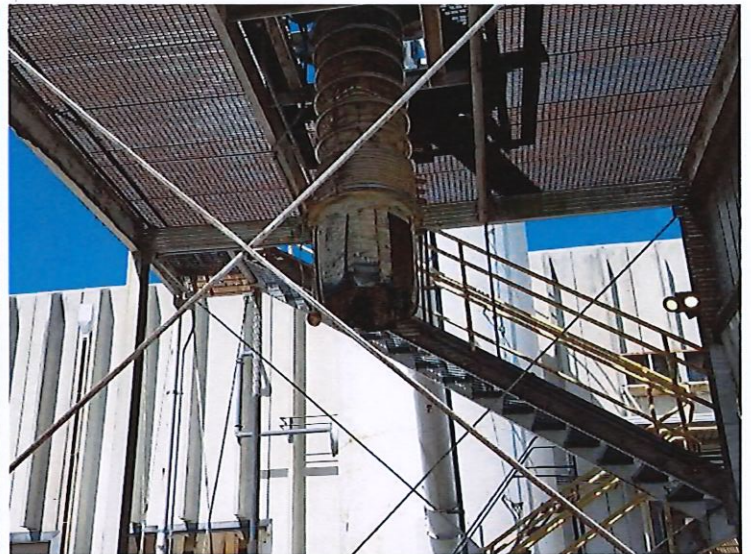
View looking up at the telescoping chute at the tissue loadout (EP-23).
