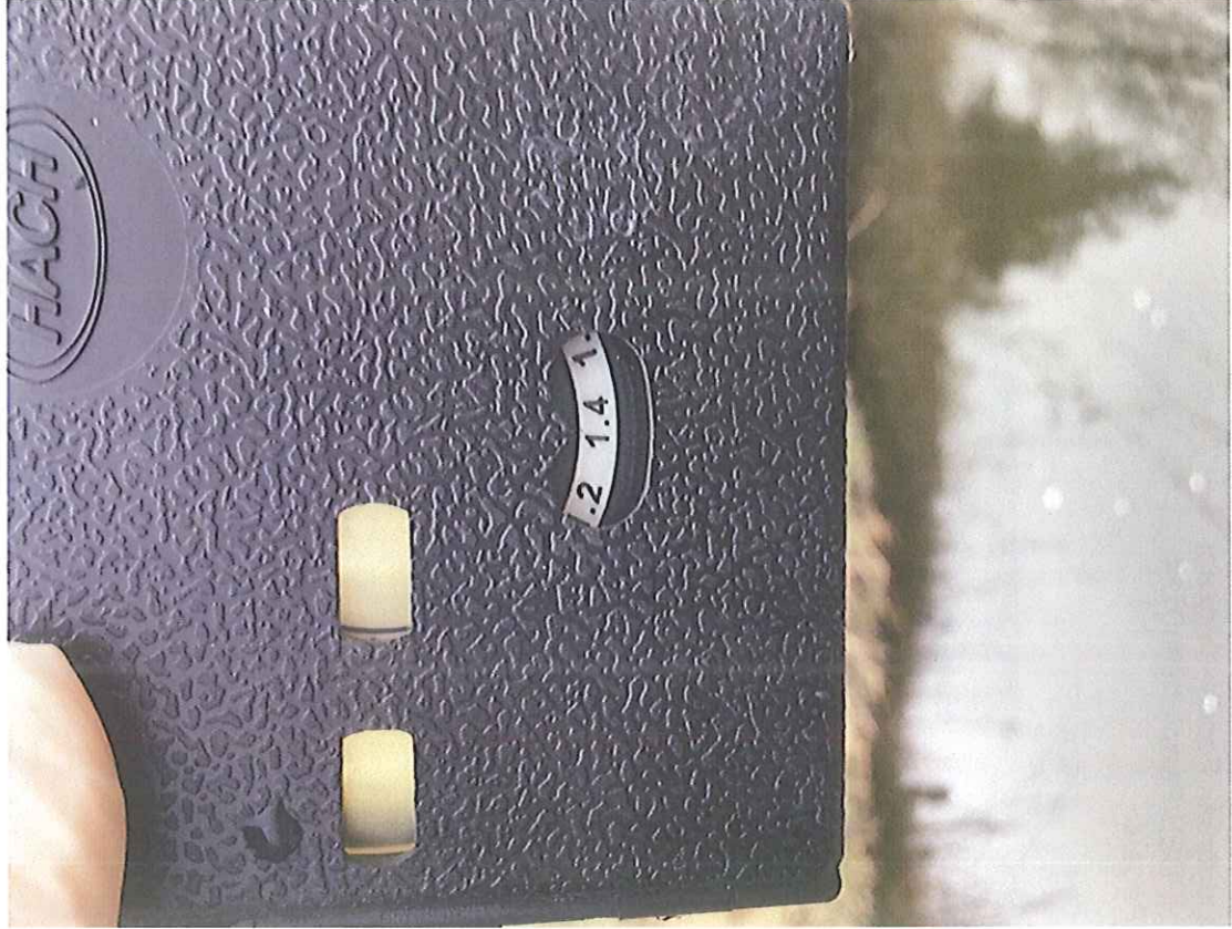
Hach Field Test Kit ammonia results at 310 th and Buchanan sample location. Ammonia concentration of 1.4 mg/L observed. (5/02/2018)
