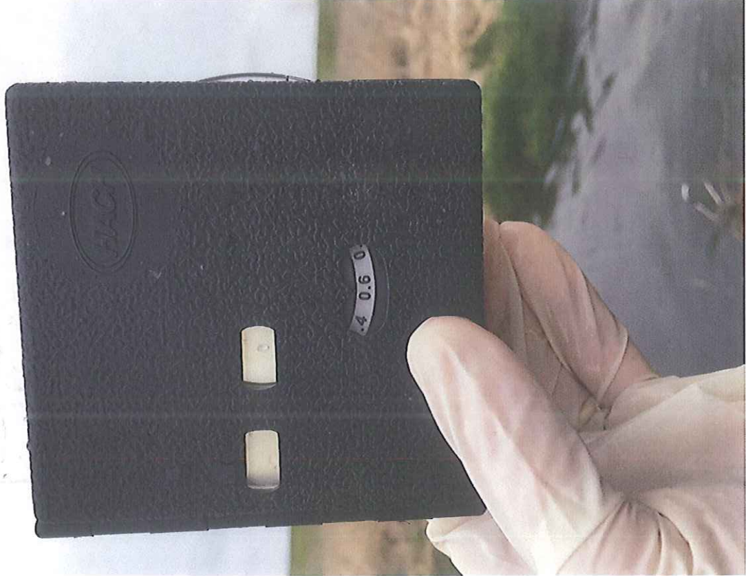
Hach Field Test Kit ammonia results at 310 th and David sample location. Ammonia concentration of 0.6 observed. (5/02/2018)
