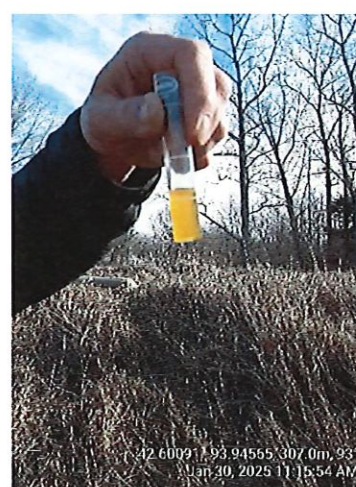
HACH sample of STW pond still >3 mg/L ammonia taken on 1/30/2025.
