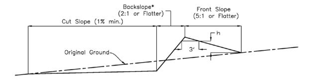
Length of front slope shall be in increments of machinery width but not less than 15 feet
