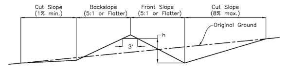
Length of front slope and backslope shall be in increments of machinery width but not less than 15 feet h = Design height of the terrace
