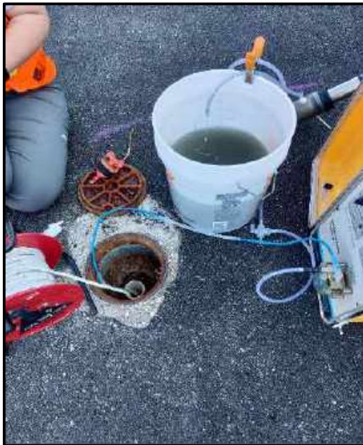
Photo 5: A Stantec crew member taking groundwater parameters out of MW-17.
