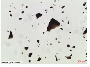
The sample was also examined with SEM/EDS, as shown below. Again, the particles appeared to break in a brittle manner, with sharp angular edges and conchoidal fracture lines readily visible. They were comprised primarily of carbon, with low oxygen and sulfur also present. This is consistent with coal.
