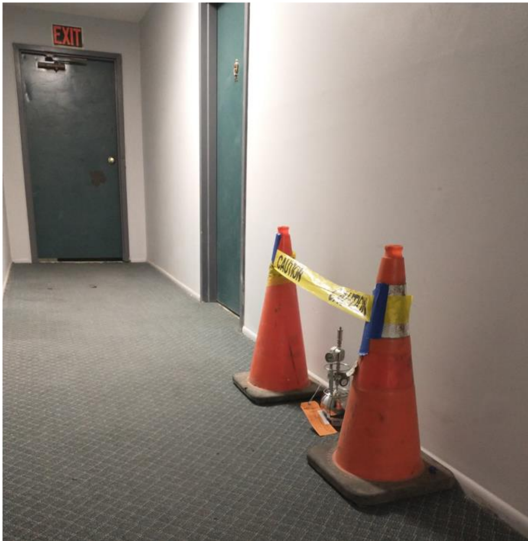
Picture 1: Summa Canister placed in the Hallway of the Apartment @ 810 Payton Ave, Des Moines, Iowa.
