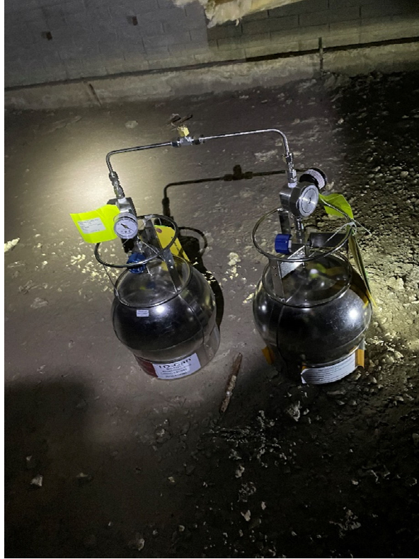
Photo 7: View of sampling train for Central sample and duplicate.
