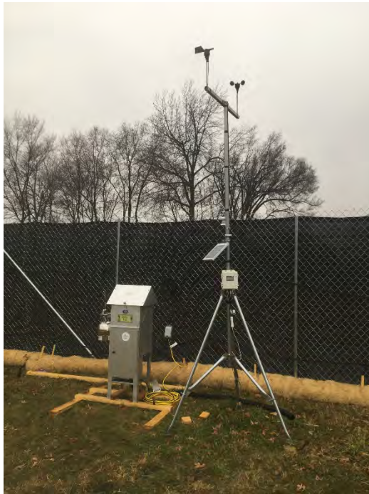
Photo 3 – Data-logging meteorological station and one of four air sampling stations for BTEX and PAHs (facing NW).
