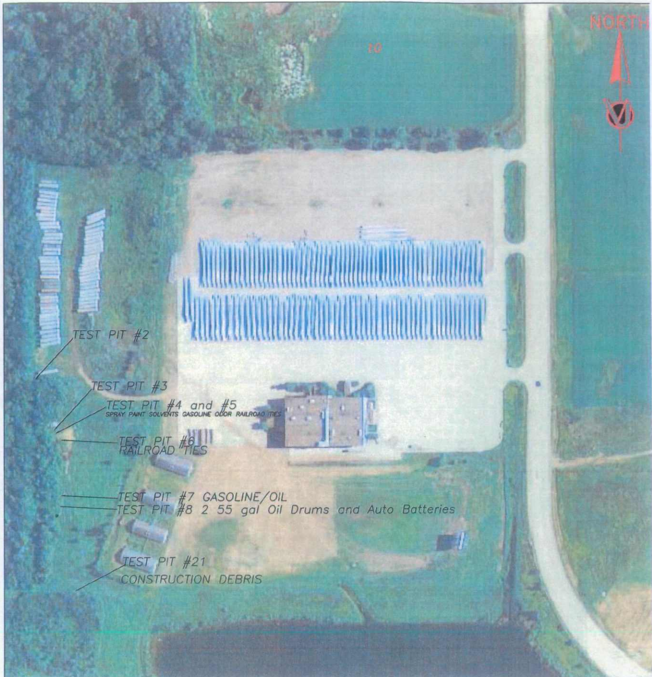
TEST PIT #2 OIL DRUM mixed with garbage TEST PIT #3 2-5 gallon paint containers (full) motor oil and paint thinner containers TEST PIT #4 and #5 Spray Paint Cans and Railroad Ties TEST PIT #6 Railroad Ties TEST PIT #7 Gasoline/Solvents TEST PIT #8 Gasoline Smell/55 gallon oil drum and car batteries TEST PIT #21 Demolition Debris FIGURE 2: SITE PLAN MAP
