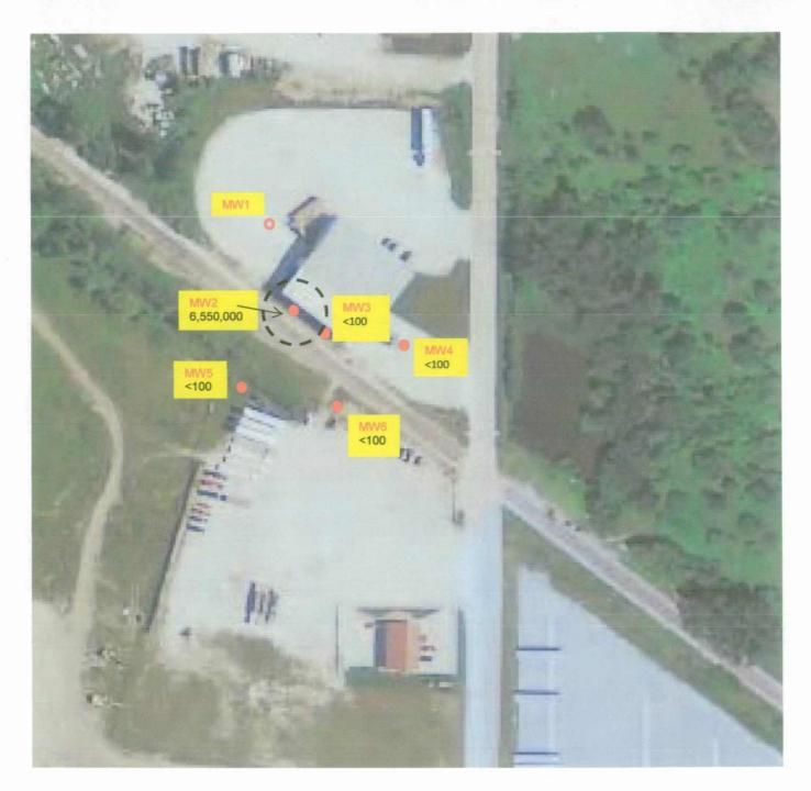
TEH diesel was detected, above IDNR target levels, in only MW2. Levels in ug/l are shown at MW2 where diesel was detected. An approximate plume encompasses sites above IDNR target level.
