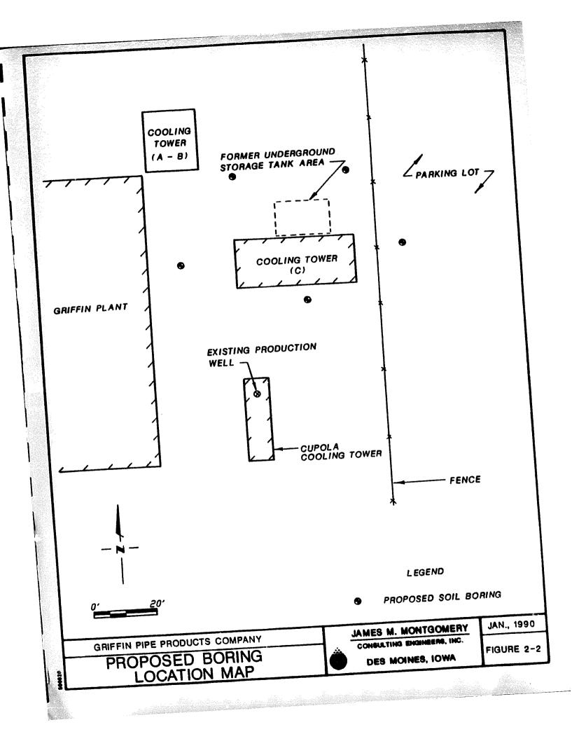
into monitoring wells will be sampled and then backfilled with bentonite and hydrated. Prior to drilling, all underground utilities at the site will be located and recorded. If the proposed placement of a boring threatens to contact any of the identified utilities, JMM personnel on site will relocate the boring in an area which will still yield substantive data.
