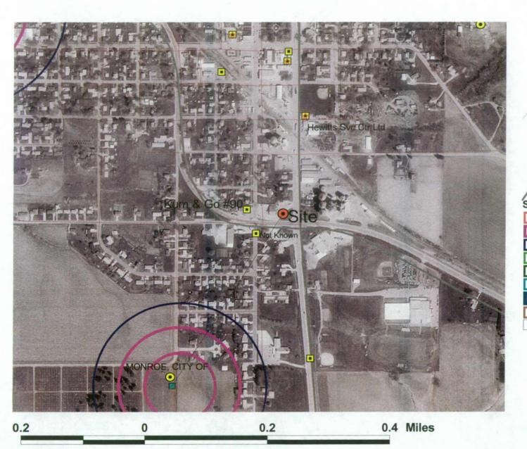
Roads\_2000\_50.shp Municipal wells LUST sites **UST Sites** Welltest Geologic sampling points.shp **Pvtperm** Highway.shp Source Water Protection Area 2-year 5-year 10-year 2500-foot 1-mile primary protection area surface runoff area hydrologic boundary
