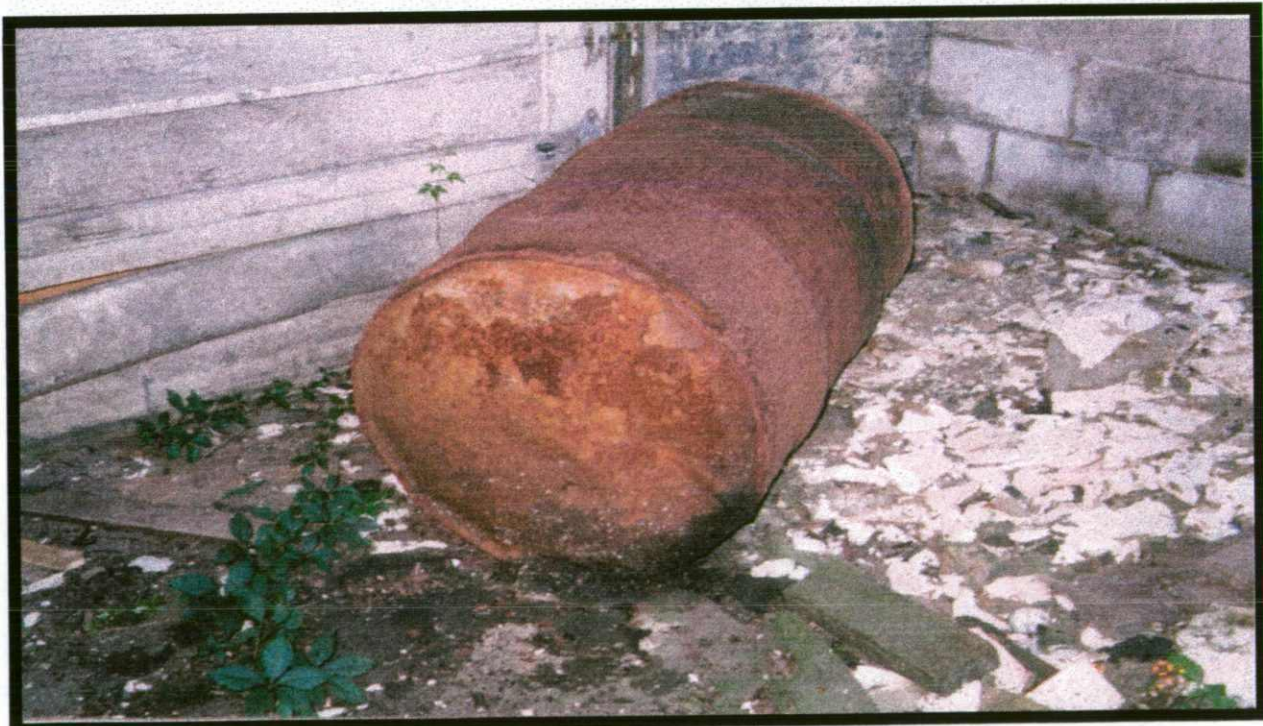
Heavily corroded 55 gallon barrel with noticeable staining. Appears to be empty. Assumed to have contained petroleum product. Located along the south wall of the southwestern portion of the site.
